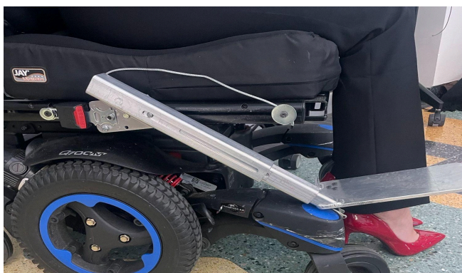
Figure [7]: Right side view of the footrest fully retracted and locked
