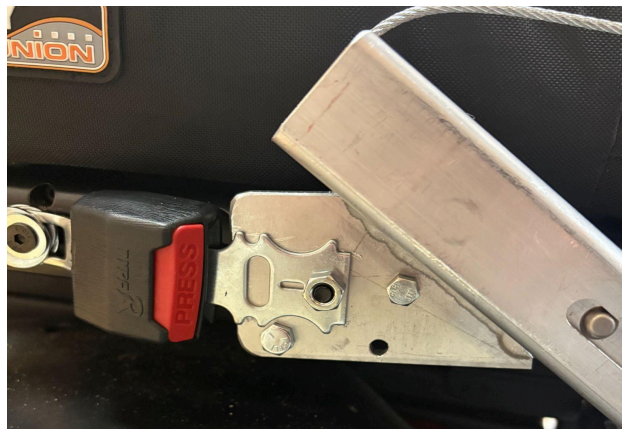
Figure [6]: Enlarged view of the locking mechanism on the left footrest.
