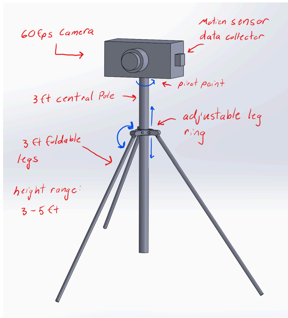
Figure 1. Motion System Design. A camera will be set up to track direct movement of the user, and this data will be recorded.
