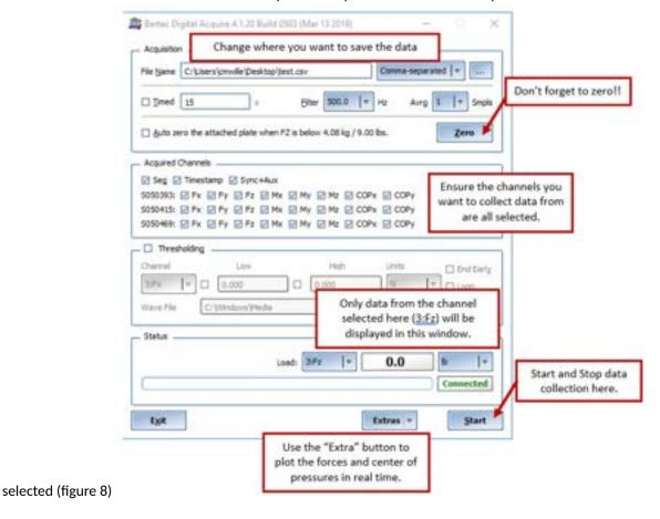
Figure 8. Annotated user interface for Bertec Acquire 4.
