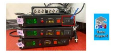
**Figure 1. A.)** Amplifier boxes for the in-ground force plates. The blue arrow indicates where the power switch is. **B.)** Bertec Acquire 4 software for data collection of force plate data.
