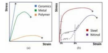
NiTi is the most effective material choice for self-expanding stents since the material choice must be able to undergo large deformation and have a low elastic modulus. → allows for a crimp into a sleeve for delivery
