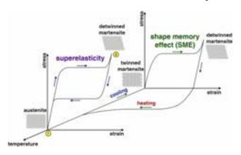
Superelastic mechanical properties of NiTi are only evident within the temperature range between the austenite finish and determined martensite deformation temperatures
