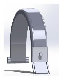
Figure 4. SolidWorks model of headband
