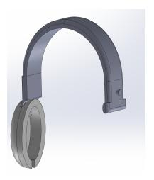
Figure 1. SolidWorks model of final design, interior of earmuff included
