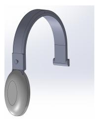
Figure 2. SolidWorks model of final design, exterior of earmuff included
