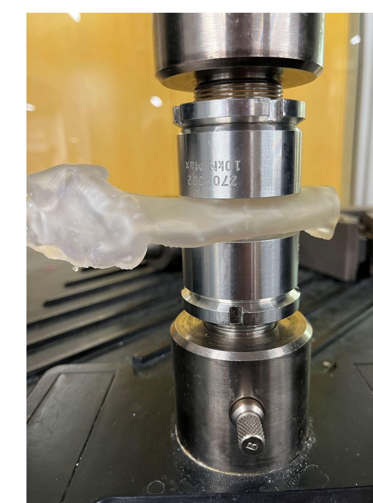
Figure 12: Flexible Resin After Compression
