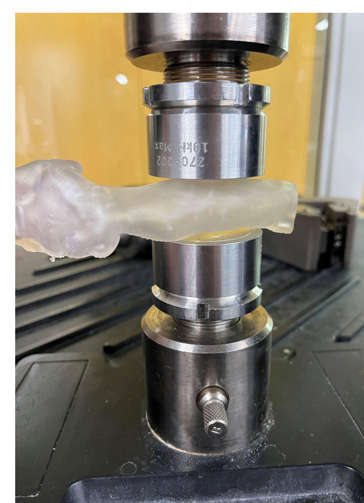
Figure 11: Flexible Resin Before Compression
