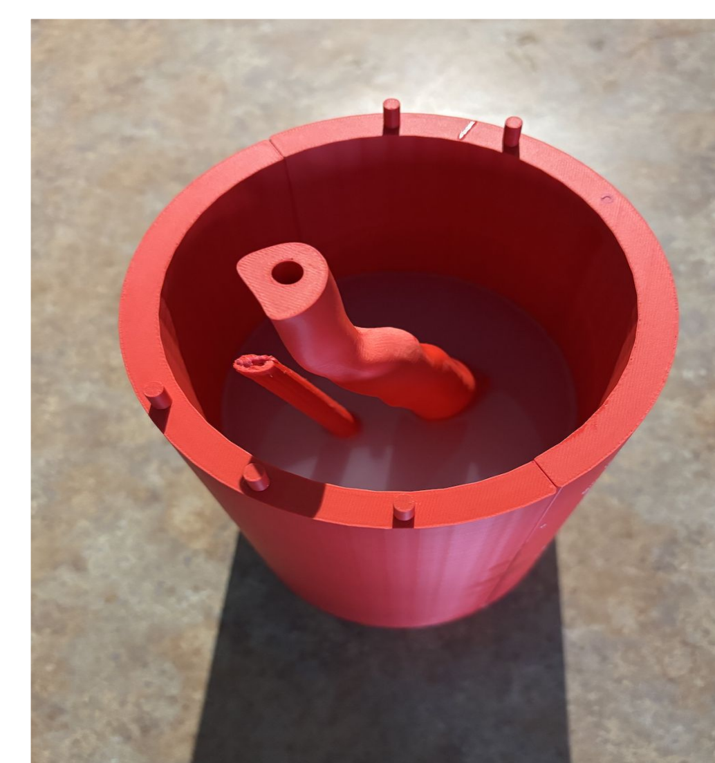
Figure 8: Silicone Mold Casting
