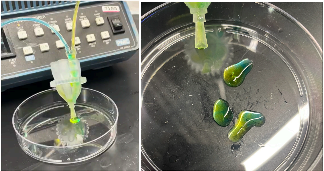
Figure 16: Testing pushing two different colored gelatins through the CEVIC and IRE (left) and the resulting hydrogels (right)
