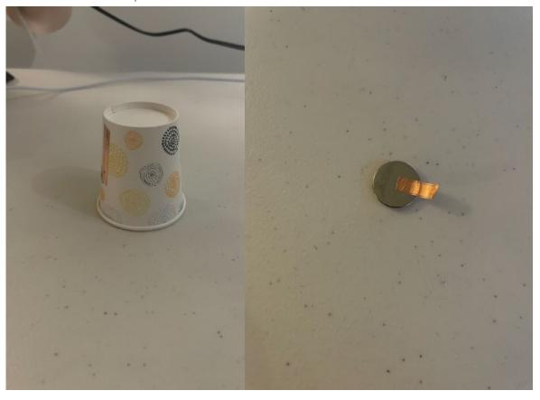
3) Place the taped side of the battery down on the top of the cup. Let the copper tape go over third piece the edge and align with one of the copper strips on the cup.
