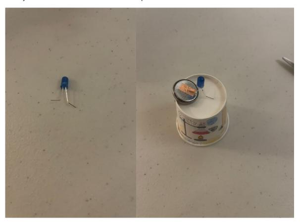
7) Take a longer piece of copper tape and wrap 8) Take one wire and identify the part of the wire it around the **positive** (longer) leg of the LED where it is stripped (no plastic) and connect it to the other piece of copper tape.
