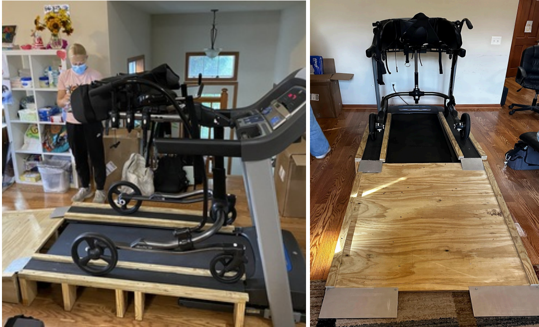
Figure 1: The Fall 2024 fabricated design features wooden side rails for the gait trainer to rest on top of with a wooden ramp leading up to the treadmill. The images above feature the patient's Rifton Pacer Gait Trainer with the K640 Large Utility Base. The wooden side rails are built to rest above the side of the treadmill and laterally extend the usable area for the Gait Trainer to rest.
