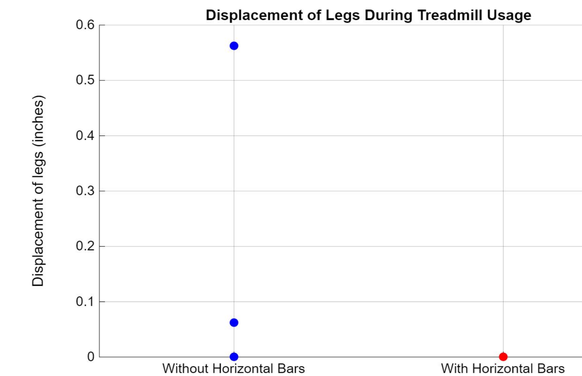
Figure 8. Displacement of side rail legs during device use
