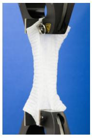
Citation: [1] ASTM D5034–21, Standard Test Method for Breaking Strength and Elongation of Textile Fabrics (Grab Test), ASTM International, West Conshohocken, PA, 2021.
