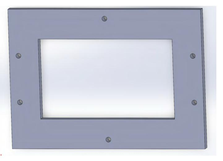
The front panel is relatively simple. The outer dimensions perfectly match the enclosure to ensure that aesthetically it looks very solid. The inner dimensions were calculated by using the bevels in the touchscreen/black areas of the screen to ensure that there is actually enough coverage of the front panel on the touchscreen. The hole locations also perfectly match the enclosure. Below the dimensions for the front panel can be found.
