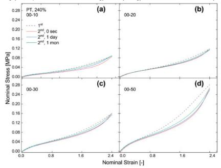
Above: Time dependence of the stress recovery under a planar tension mode at strains of 240% for different Shore hardnesses. The second loading paths with recovery times of 0 second, 1 day, and 1 month (solid lines) compared with the first loading paths (dash line) for Shore hardnesses (a) 00-10, (b) 00-20, (c) 00-30, (d) 00-50, are presented, respectively.
