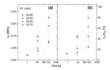
Above: The time dependence of the dissipation during the second cycles of planar tension tests at strains of 240% for Shore hardnesses 00-10, 00-20, 00-30, 00-50. (a) The subsequent softening dissipation energy density, (b) the softening dissipation ratio between the subsequent and initial softening dissipation energy density
