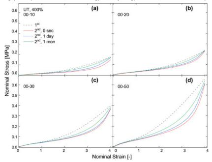
Above: Time dependence of the stress recovery under a uniaxial tension mode at strains of 400% for different Shore hardnesses. The second loading paths with recovery times of 0 second, 1 day, and 1 month (solid lines) compared with the first loading path (dash line) for Shore hardnesses (a) 00-10, (b) 00-20, (c) 00-30, (d) 00-50, are presented, respectively.
