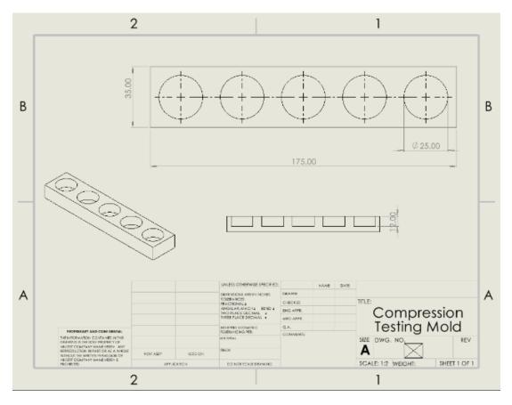
Mold for compression testing of the ecoflex
