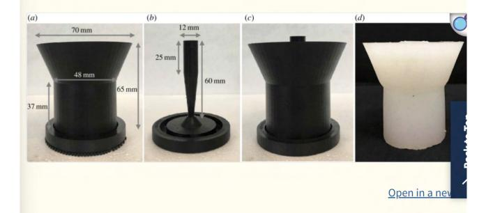
Panel (a) shows the outer piece of the cervical mould; (b) shows the inner section of the cervical mould used in these experiments. Panel (c) shows the outer and inner pieces assembled into one and (d) shows the resulting silicone model removed from the mould after curing. (Online version in colour.)
