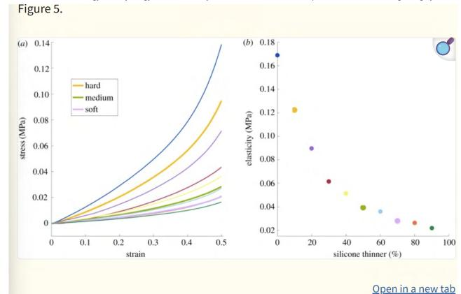
The material testing results of the silicone samples (a) The stress–strain curves for exof the 10 types of silicone tested. (b) The modulus of elasticity of the linear region is reported as a function of silicone thinner added to the sample. (Online version in cold
