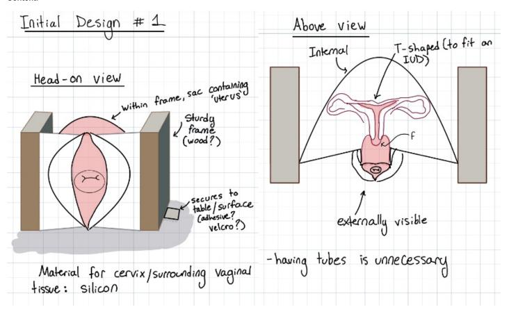
Conclusions/action items: The design needs work, and does not yet include dimensions or materials for all the moving parts. It will need more development and refinement. The fallopian tubes are also an unnecessary feature, but are included in this initial sketch.
