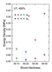
Above: The initial softening dissipation energy density (black dots) and viscoelastic dissipation energy density (red dots) of uniaxial tension tests at strains of 400% for different Shore hardnesses.
