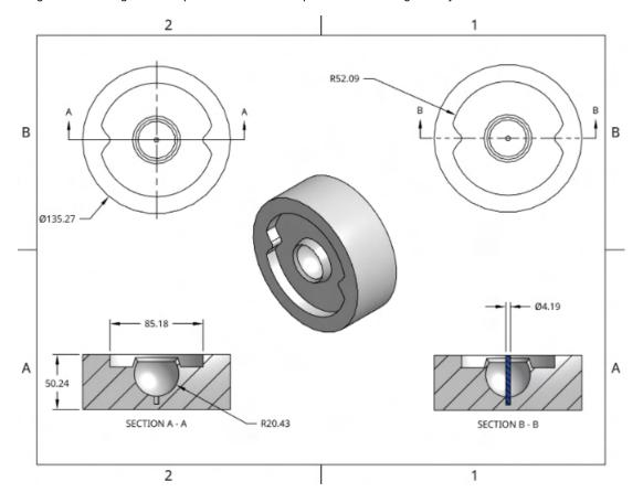
Conclusions/action items: 3D Print the new mold and then cast in silicone.
