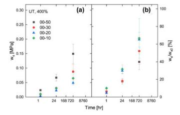
Above: The time dependence of the dissipation during the second cycles of uniaxial tension tests at strains of 400% for different Shore hardnesses. (a) The subsequent softening dissipation energy density, (b) the softening dissipation ratio between the subsequent and initial softening dissipation energy density.
