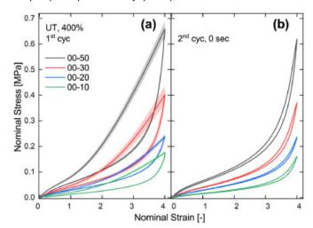
Above: Stress-strain response of the two-cycle uniaxial tension tests at strains of 400% for four Shore hardnesses 00-10, 00-20, 00-30, 00-50. (a) The first cycles with error bands, (b) the second cycles applied 0 second after the first cycle.
