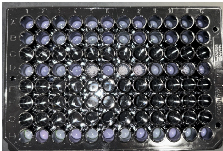
Figure 24: 96-well plate sample containing fluorescein in odd numbered columns and no fluorescein in even numbered columns
