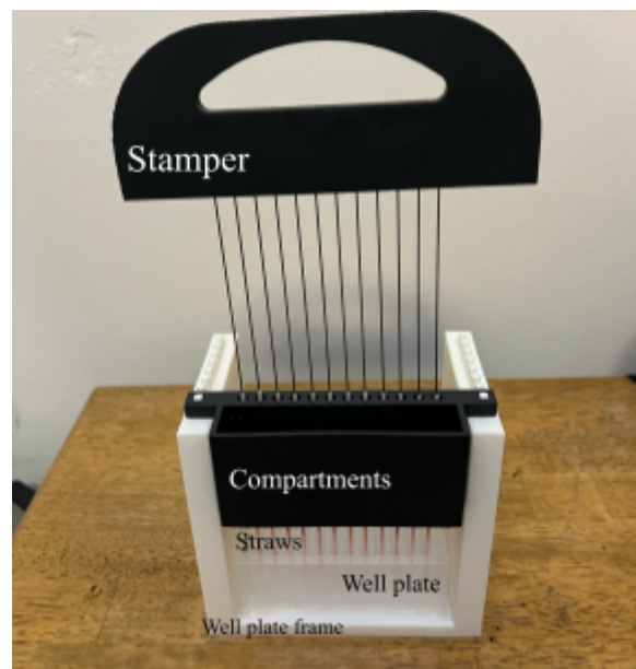
Figure 9: Final printed assembly of well plate frame, compartments, and stamper
