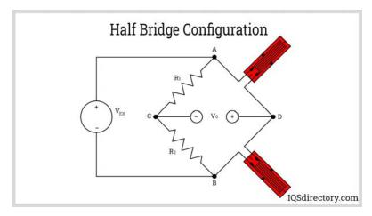
Half wheatstone bridge configuration showing strain gauges in red.
