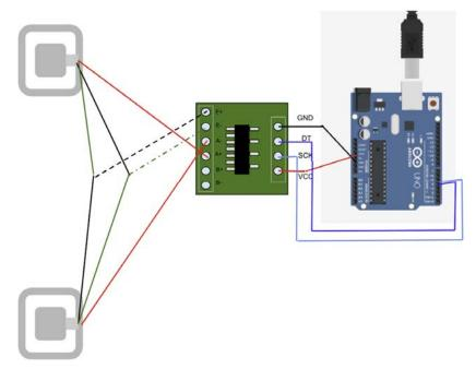
*Figure 11* Load cell circuit to Arduino [15]. The green wire is the white wire.
