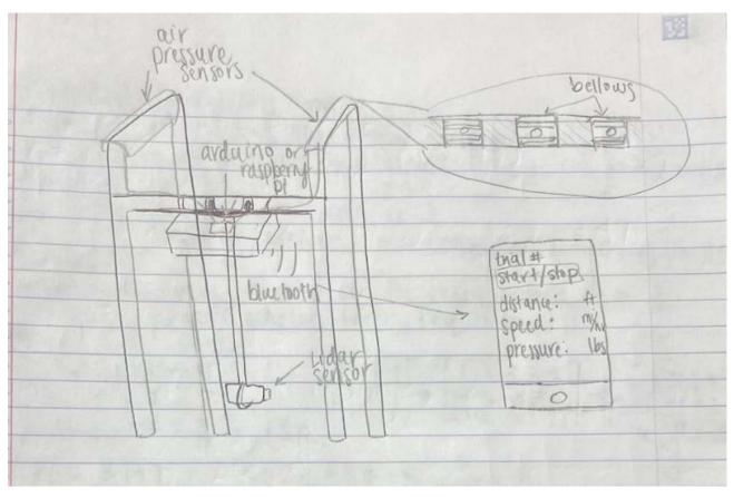
Conclusions/action items: This design will not work because squeezing the handles could impact the pressure reading.
