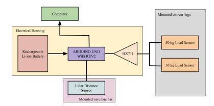
Figure 8 Circuit block diagram of design and components.
