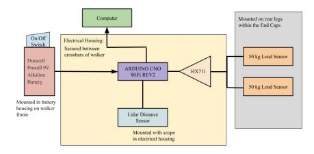
Figure 10 Circuit block diagram of design and components.
