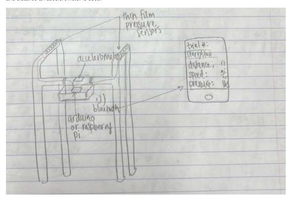
Conclusions/action items: This design will not work because squeezing the handles could impact the pressure reading and the accelerometer is less effective.
