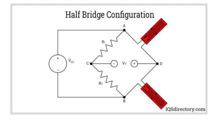
Figure 7: Half wheatstone bridge configuration showing strain gauges in red [9].
