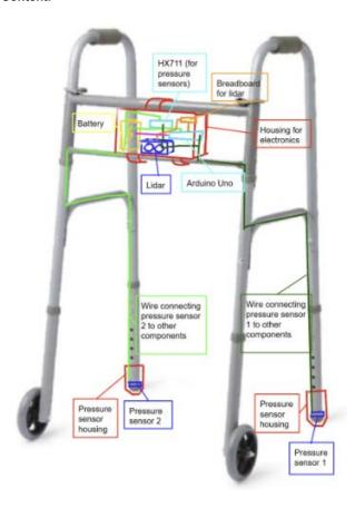
\* This image does not include a component to hold a phone or connect to Bluetooth because we have not finalized the designs on how those pieces will work.
