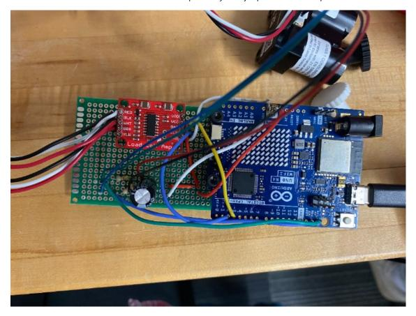
Connections were soldered directly to the arduino.
