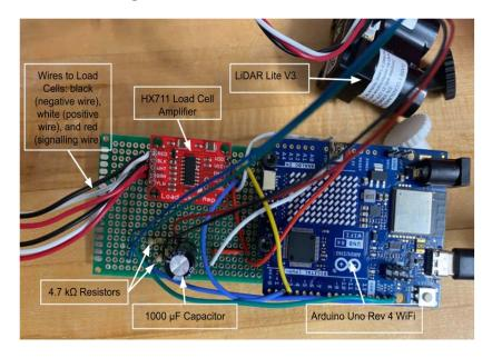
Figure 13 Complete combined circuit on perfboard
