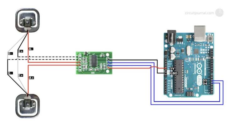
This is the image of the wiring plan that we had. We set up our circuit according to this when we met as a group to try to hook up the pressure sensor to a computer and upload code however we had issues with getting the calibration value to be correct.
