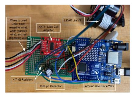
Figure 15: Complete combined circuit on perfboard
