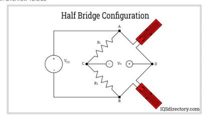
Figure 8: Half wheatstone bridge configuration showing strain gauges in red [11].
