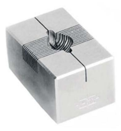
^^^ WPI Stainless Steel Rodent Brain Matrices, meant for thin and uniform brain slices. Made of durable stainless steel. Include precison cut channels to run the balde through, making 1 mm thick slices. Also available in different sizes for different species. Easily chilled and or sterilized. Stainless steel useful when heat transfer or maintaining a specific temperature range is required. \$345.00
