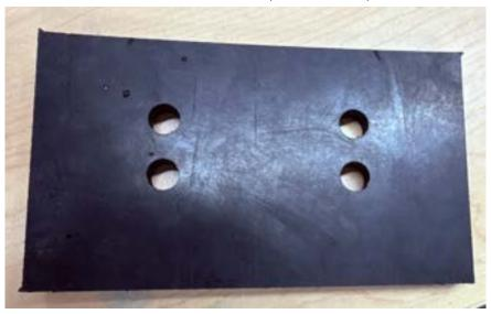
Figure 2: Finalized base design of neoprene rubber
