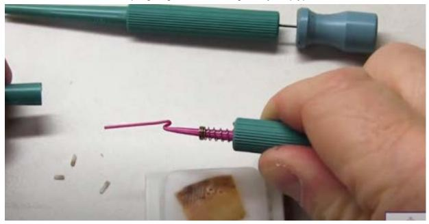
$\ensuremath{^{\wedge\!\wedge\!\wedge}}$  failure of the internal plastic plunger mechanism
