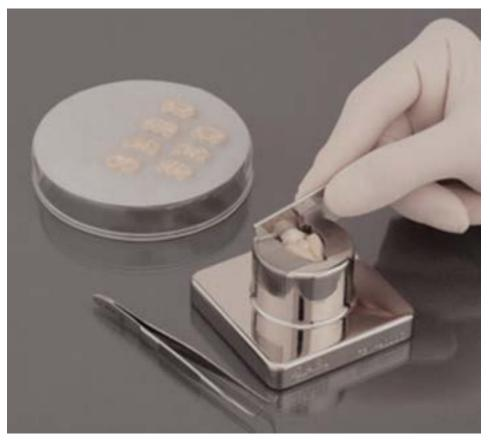
^^^ Designed to aid in freehand dissection of rodent brain. Meant for consistent and reproducable sections at varying intervals depending on item purchased, show is designed for 1 mm slices. Different models avaible for safittal cuts and coromal cuts. Cast in High Grade Zinc using the actual animal prain for cavity definition. Can be chilled and sterilized.
