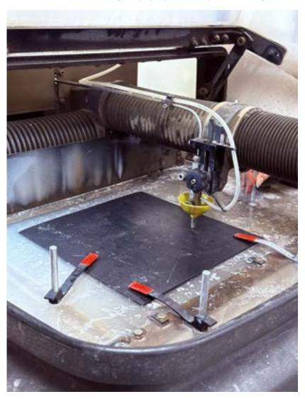
Figure 1: Fabrication of neoprene rubber base plate using waterjet cutting machine from D.I. Lab
