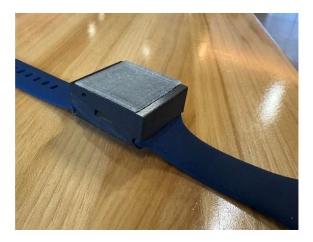
Conclusions/action items: Print resin again with supports in the slits to provide a tighter fit
