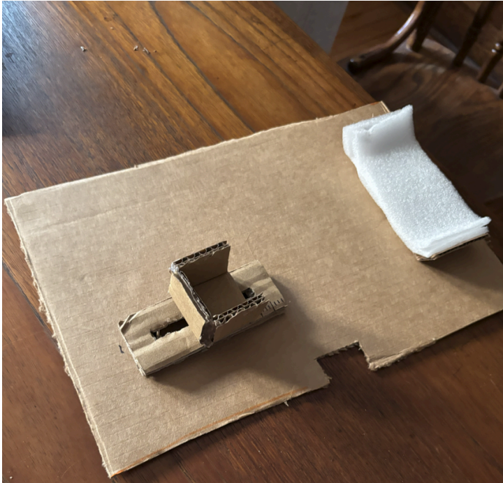
Figure 2. Rough proof of concept prototype featuring a singular finger track and slider.
