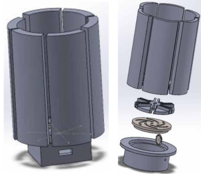
Figure 10. (A) Side view of Expanding Pulley System CAD model. (B) Expansion of CAD model.
