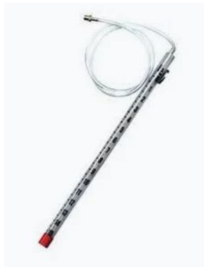
Figure 22: Water manometer example [27]
