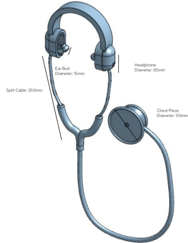
Figure 6: Headset CAD design [5]
