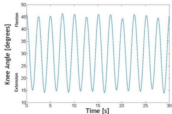
**Figure 7: The repeatability of the knee angle over 12 cycles: Average range of motion was  $45.5^\circ \pm 1.04$  (max) and  $14.6^\circ \pm 0.85$  (min).**
