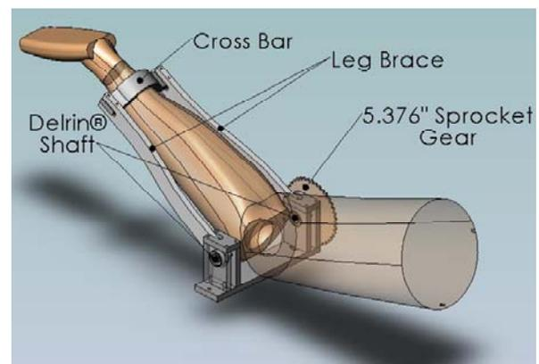
**Figure 5: The leg support assembly.**
