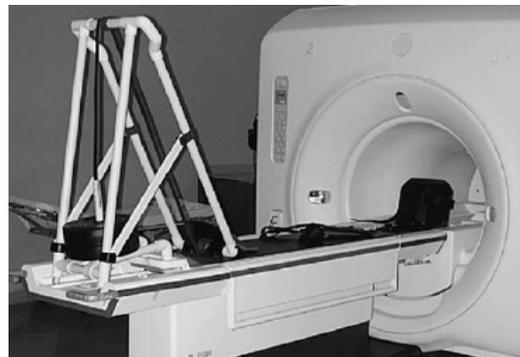
Figure 1: Weight bearing apparatus to measure knee contact area.
