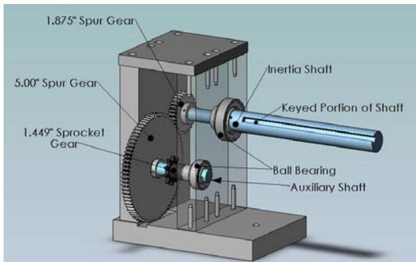
**Figure 6: The gear box of the inertia loading system.**
