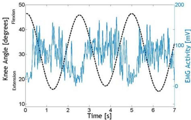
**Figure 8:** This graph shows the EMG data of hamstring activation superimposed with the cycle of motion during inertial loading. The hamstrings become most active when the knee is fully extended.
