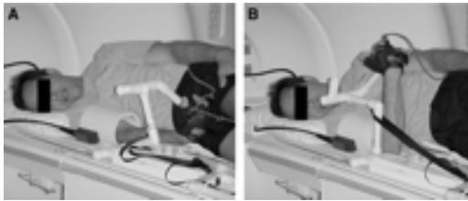
**Figure 2: Elastic load device for measuring biceps velocity.**
