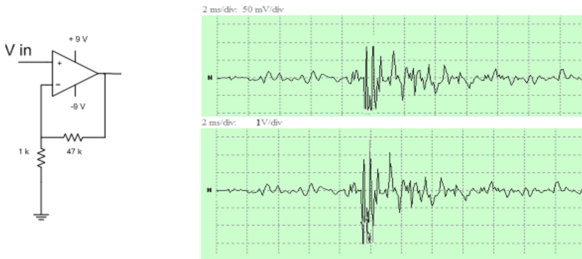
Figure 5: First stage voltage amplifier. Notice how the sample output waveform (bottom) is simply the amplified version of the sample input waveform (top).
