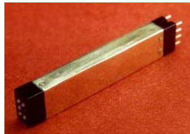
Figure 7: Microsolenoid driven Braille cell, used by researchers at MIT. http://web.mit.edu/erblan/www/Graphics/solenoid-big.jpg
