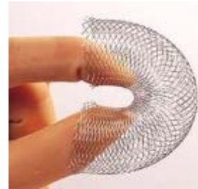
Figure 6: Smart metal alloy, shown as a deformable stent. It has many other applications in medical technology for its flexibility and “memory” abilities. http://www-civil.eng.ox.ac.uk/people/zy/research/stent.jpg
