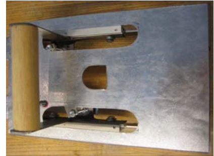
Figure 10 - Top most metal sheet showing hole for pill as well as tracks cut out for advancement of bracket/blade assembly
