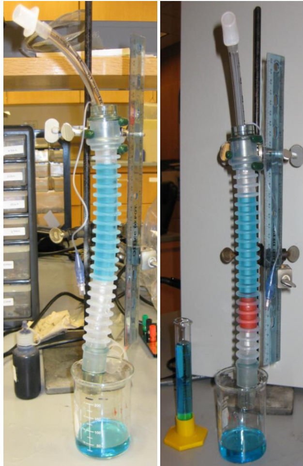
Figure 6: Testing apparatus simulating trachea full of subglottic secretions without (left) and with (right) cuff wrapper
