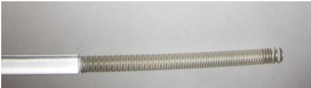
Figure 3: Insertion tool with both coils wrapped around it. Notice the constant pitch of the coils and the clear plastic between every rung
