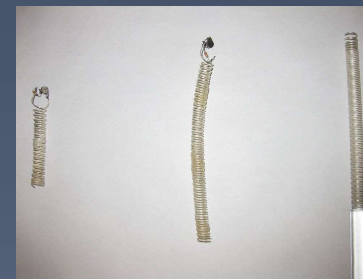
Figure 2: Two different sized current coils (left and center) and a coil attached to insertion tool (right)
