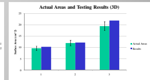
Chart 3: 3D System Testing The green bars represent the area of each shape calculated based on planar geometry. The blue bars represent the average of the system's calculations based on images of the shapes in various three dimensional configurations. Error bars are +/- 10%.
