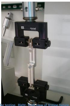
Figure 4: Left-side view of testing fixture with acrylic cap in place for testing. Right- iron view of testing fixture camped into tensile tester with acrylic cap in place for testing.
