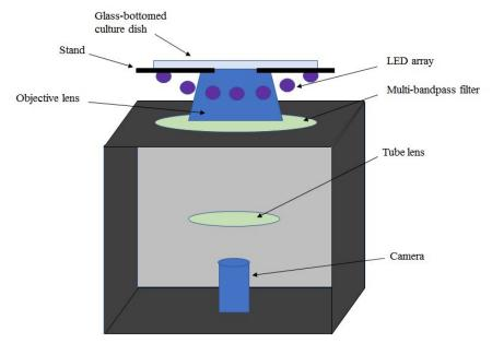
FIGURE 4: Single-Shot Design Schematic. This is the first design idea proposed and it consists of no moving parts.
