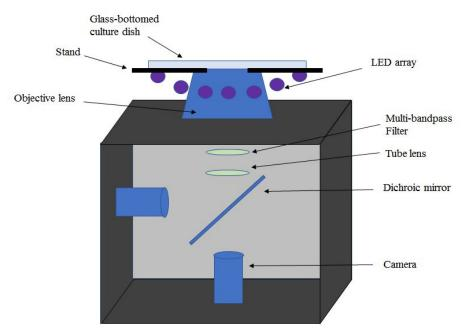
FIGURE 6: Beam-Splitter Design Schematic. This is the third proposed design and it consists of mirror that splits the two wavelengths of interest.
