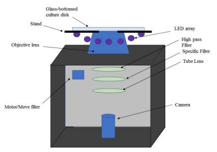
**FIGURE 5:** Filter-Swap Design Schematic. This is the second design idea proposed and it consists of a motor that swaps out the filters.
