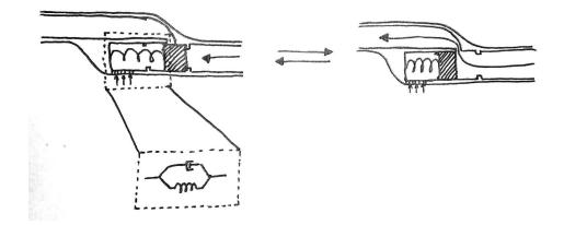
Figure 5: Spring-Dashpot operated valve. Valve is opened by inflow pressure, the movement of which is resisted by the dashpot element.
