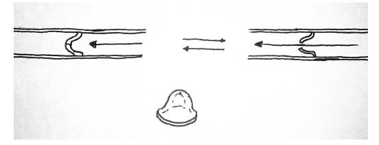
Figure 7: Differential pressure valve. Inflow pressure deforms the flexible material, expanding a small hole in the tip, allowing drainage.
