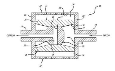
Figure 4: Differential pressure valve. Inflow pressure pushes against ambient pressure to open and close the valve.
