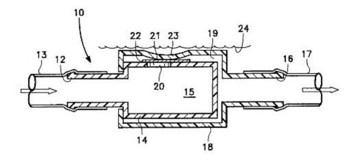
Figure 6: Ambient pressure operated valve. Inflow pressure acts against ambient pressure to operate the opening and closing of a small flap, which seals the drainage hole.
