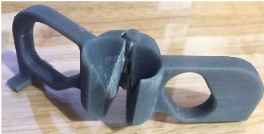
Figure 3. Grey Pro SLA resin 3D printed and assembled prototype of needle-guide.
