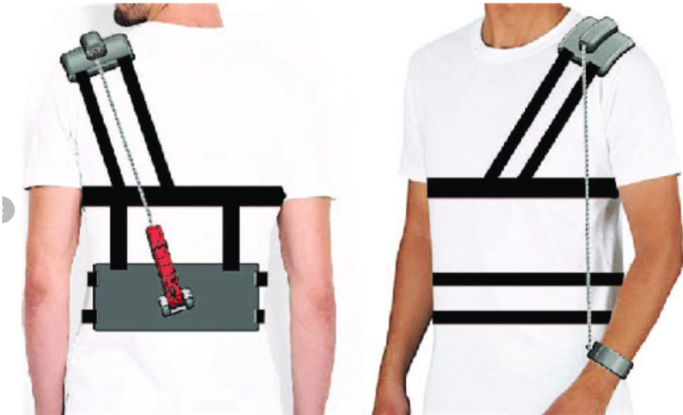
Figure 1. Motor powered elbow assistive device
