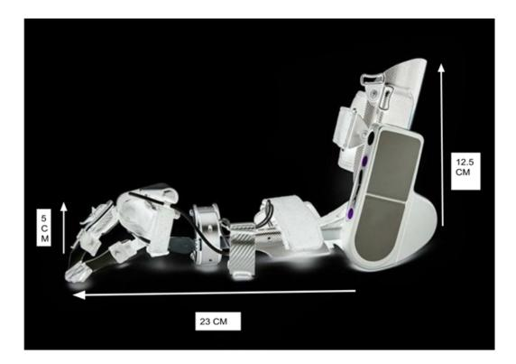
Figure 1. Mind-controlled Exoskeleton to support arm motion with signals sent from the brain. It consists of a non-invasive sensing system and an EMG signal processing system.
