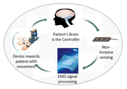
Figure 1: A brief process of how the brain can control an arm brace.
