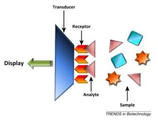
Figure 2: Schematic showing important components of a typical sensor.
