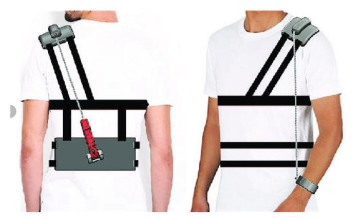
Figure 1. Motor powered elbow assistive device
