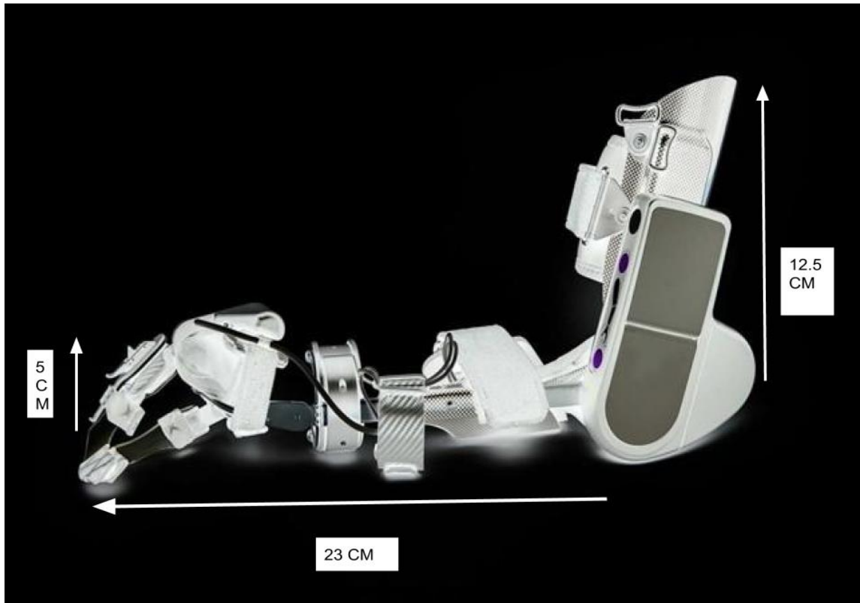
Figure 5. Mind-controlled Exoskeleton to support arm motion with signals sent from the brain. It consists of a non-invasive sensing system and an EMG signal processing system.
