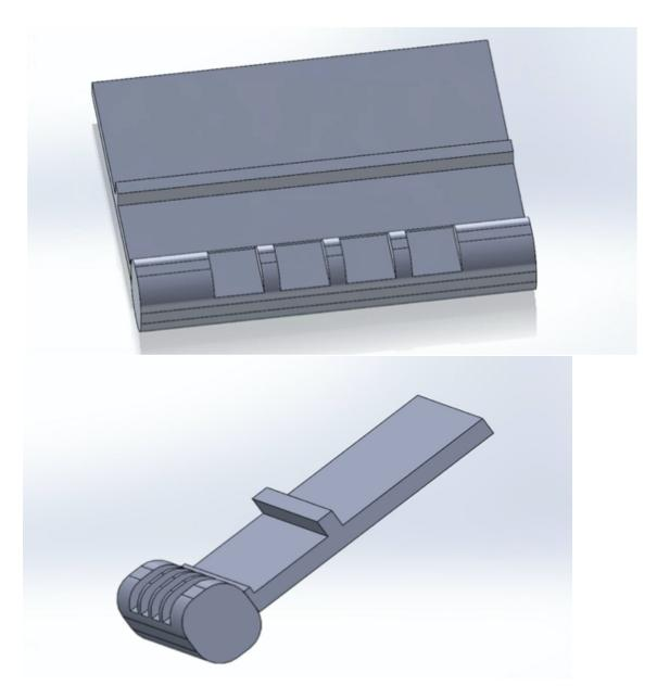
Figures 1 & 2: Updated SolidWorks design of the pinch grip.
