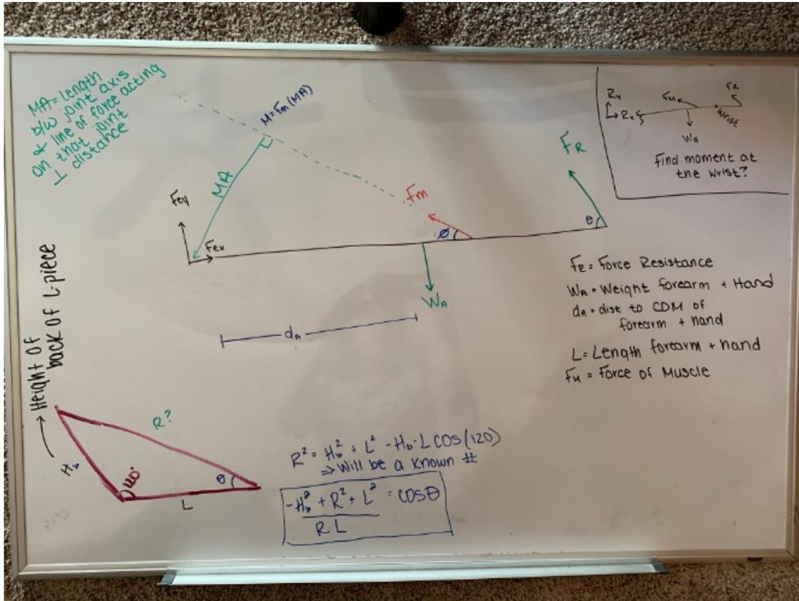
Figure 1. Rough sketches of the free body diagram of the lower arm as well and trig equation for angle of resistance band
