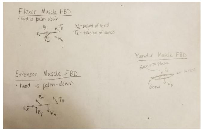
The reaction forces on the FBDs will cancel. The only forces we are really concerned about are the tension in the bands ( $T_B$ ) and the force generated by the muscle ( $F_m$ ). The moment arms give me the ability to calculate the moment generated about the wrist from the muscle that will counter the moment generated from the tension of the bands. The tension in the bands will be calculated based off of the tension tests we plan to do as a team.
