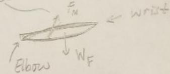
The reaction forces on the FBDs will cancel. The only forces we are really concerned about are the tension in the bands ( $T_B$ ) and the force generated by the muscle ( $F_m$ ). The moment arms give me the ability to calculate the moment generated about the wrist from the muscle that will counter the moment generated from the tension of the bands. The tension in the bands will be calculated based off of the tension tests we plan to do as a team.
