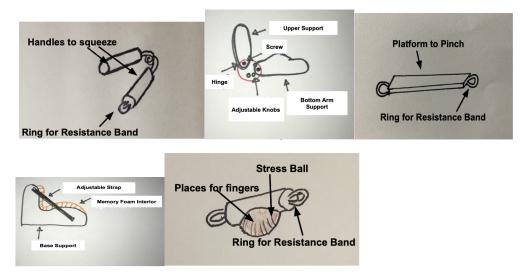
Figures 1-5: Sketches of the five preliminary designs - Gripper, Hinge, Pinch Grip, Straps, and Stress Ball Grip respectively.
