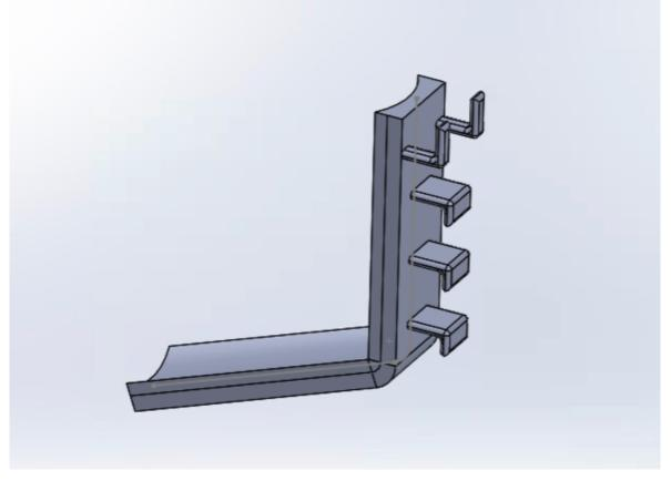
Figure 1: Drawing of L-Piece that includes an angle of 110 degrees.
