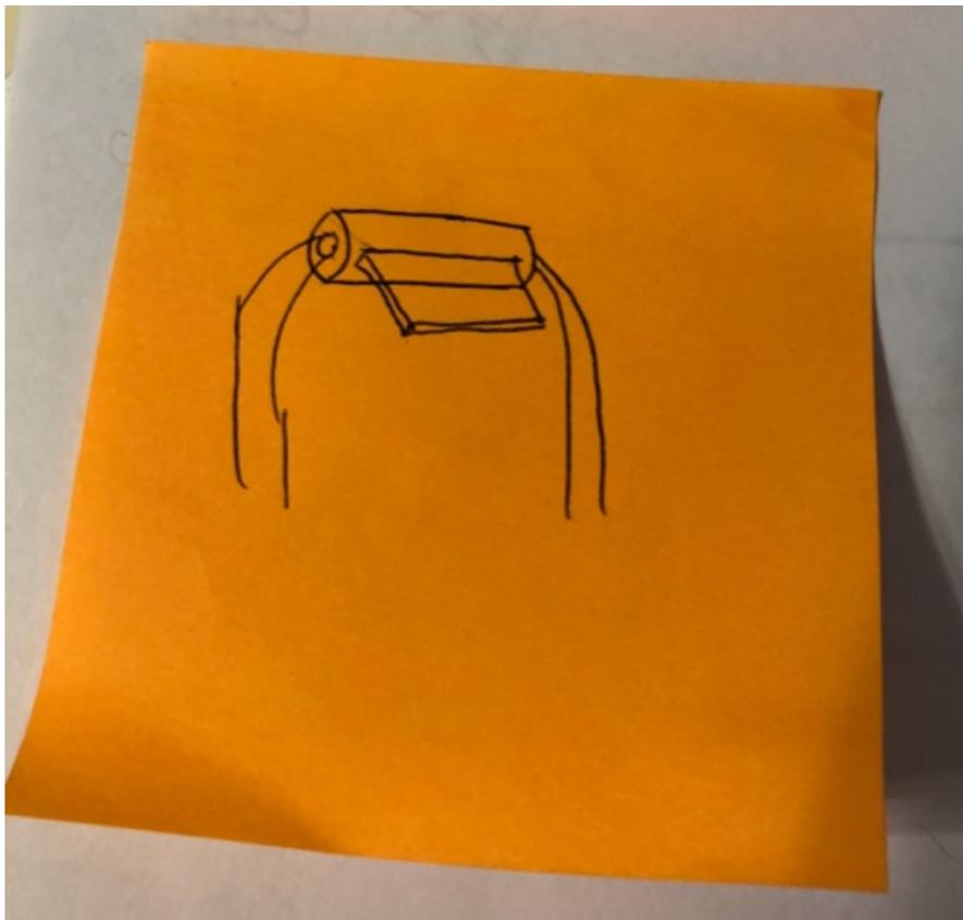
Figure 1: This is a possible design idea. It would incorporate the existing handle and band attachment, but would add a thin rectangular piece onto that to function as the pinch grip. We would need to play around with the thicknesses and the strength of attachment. to make sure it doesn't snap off.
