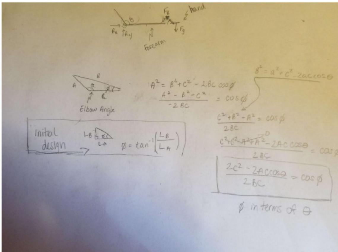
The top drawing shows the beginning of an FBD of the design with  $\theta$  being the elbow angle and  $\phi$  being the angle of the bands relative to the forearm. The boxed equation in the bottom right is an equation that represents  $\phi$  in terms of  $\theta$ . "A", "B", and "C" represent the lengths shown on the triangle in the middle of the figure.
