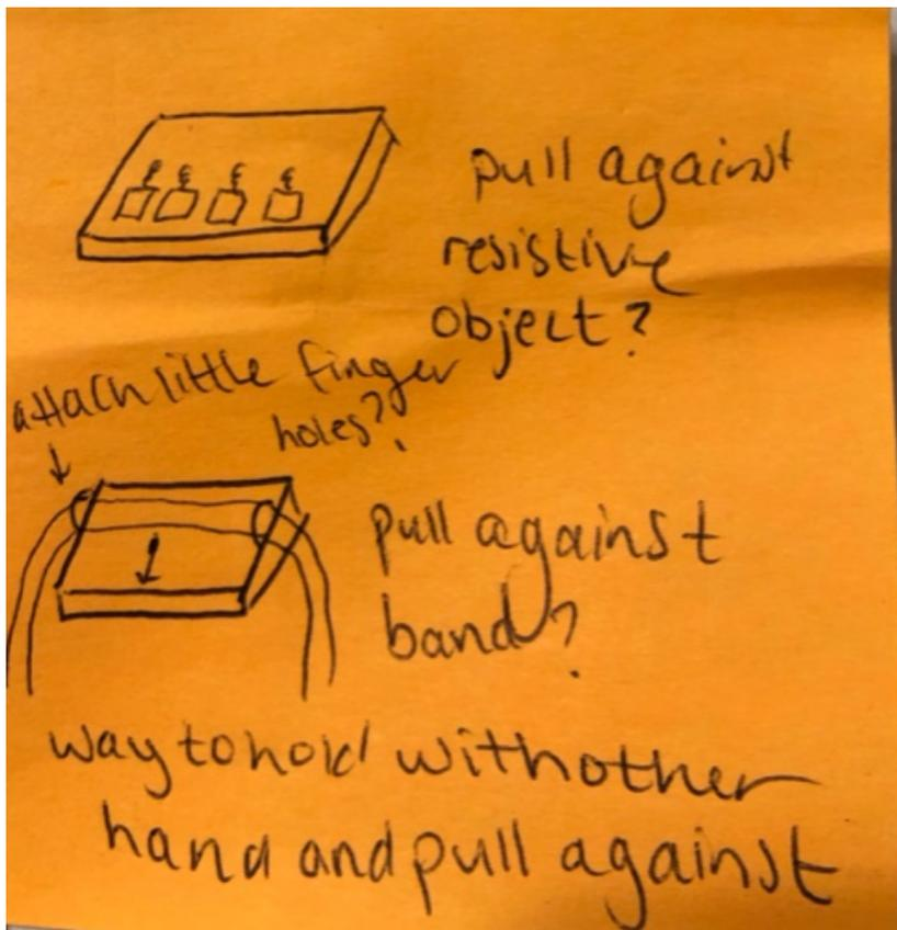
Figure 4: Another possible way to incorporate dynamic training. The band would lay on top of the pinch grip with finger holes on it, and the user could pull their fingers down the grip. This wouldn't be able to be used at the same time as the other exercises, but the static part of the pinch grip would be working the grip during those exercises anyway.
