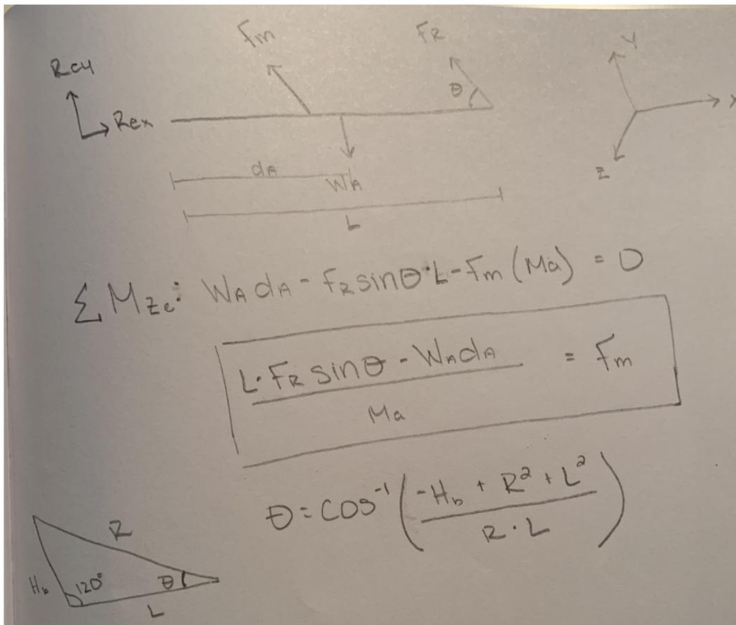
Figure 2. The equation above will work for the FBD above. It also shows the value for theta.
