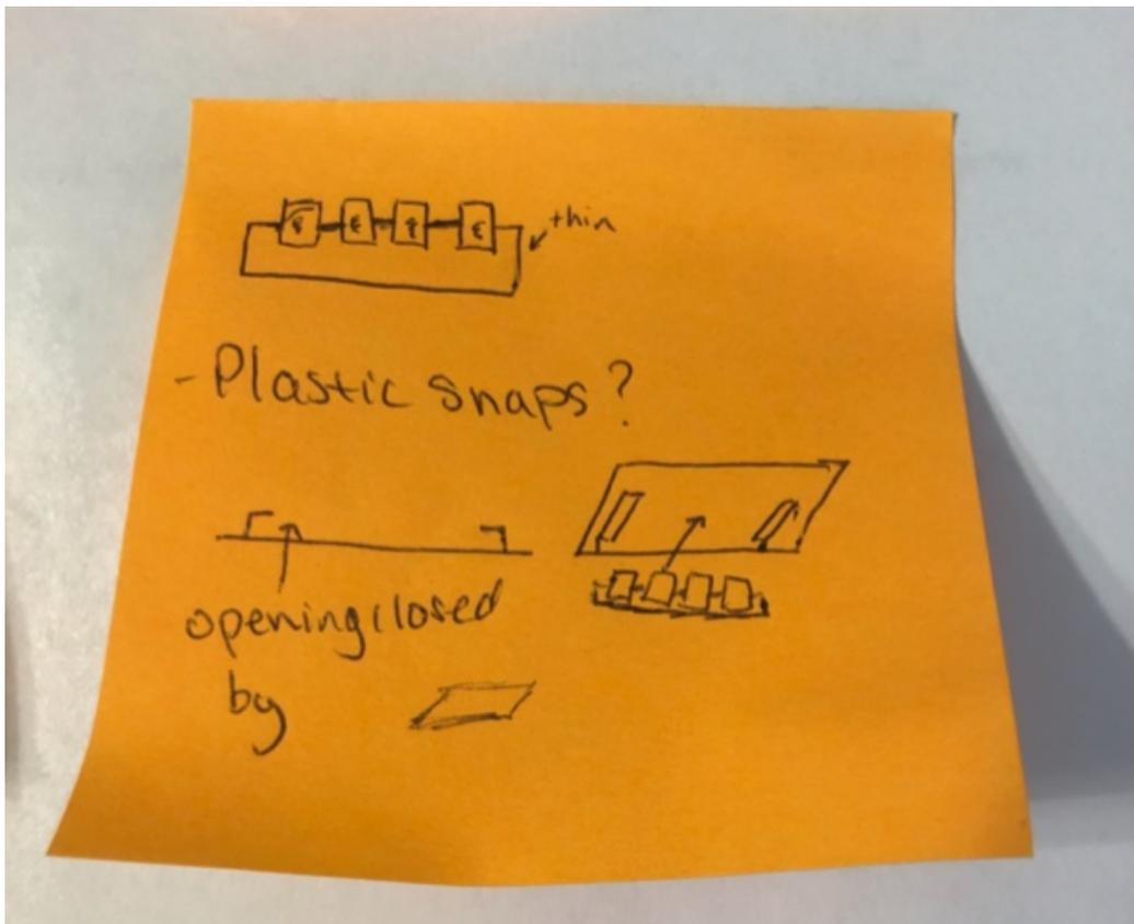
Figure 3: All of the clips could be attached onto one piece that could slide onto the pinch grip to allow for an easy way to switch them out.
