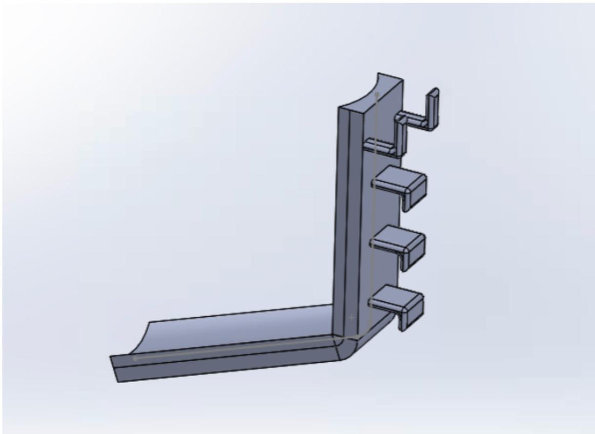
**Figure 1:** Drawing of L-Piece that includes an angle of 110 degrees.
