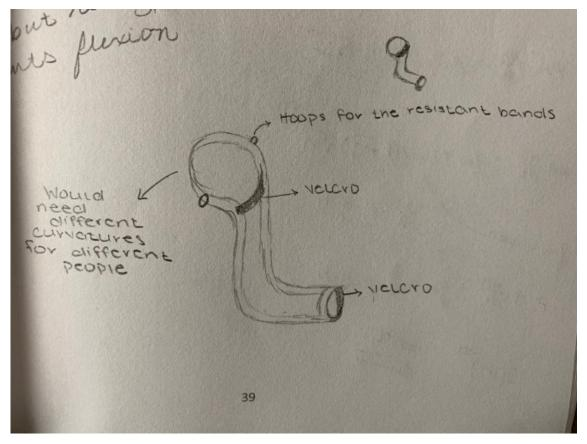
Figure 1. The brace base design.
