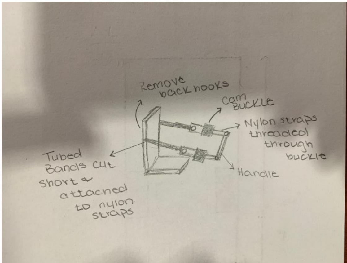
Figure 2. Drawing of the resistance band and cam buckle idea.
