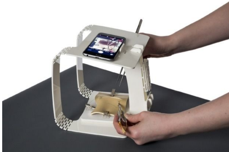
Fig. 1: eoMicro simulator. The eoMicro simulator in combination with a smartphone creates a home microsurgical set-up that allows microsurgical skill improvement [3]
