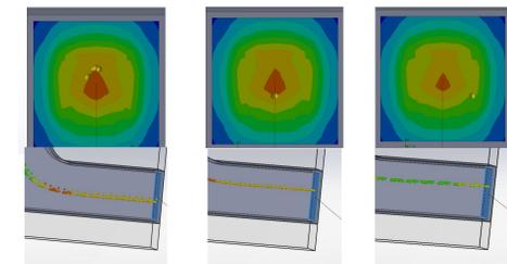
Figure 7. Cross-sectional flow velocity with side-view displayed below. Images are taken from 100um wide Snake channel at input pressures of 1, 30, and 100 mBar.
