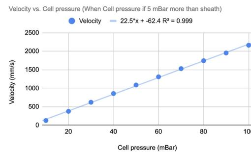
Figure 4. Graph of particle velocity in mm/s in relation to the pressure of the cell input.
