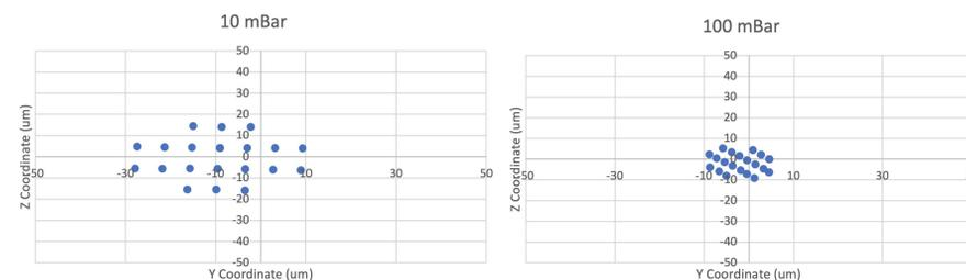
Figure 6. Graphs of the particle positions at the end of the funnel design for 10 mBar (left) and 100 mBar (right). The origin of the graph is the center of the output channel.
