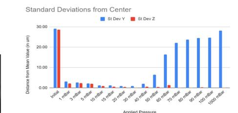
Figure 10. Standard deviations for Y and Z positions of the relevant input pressure simulations. Focusing reached its optimal level for both directions at 30 mBar (0.86 and 0.16 um in the Y and Z directions respectively).
