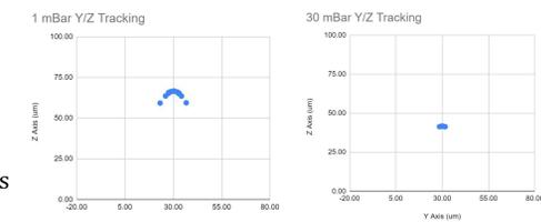
Figure 8. Y-Z Trajectory plots of particles that reached the end of the 100 um Snake channel. Focusing in both directions was most uniform at 30 mBar of pressure and started to show clear signs of divergence in the Y-direction starting at 60 mBar.
