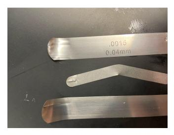
Figure 5: 0.0015 in feeler gauge, 0.0015 in toffelmier bands, and 0.002 in feeler gauge (top to bottom) post testing in MTS machine.
