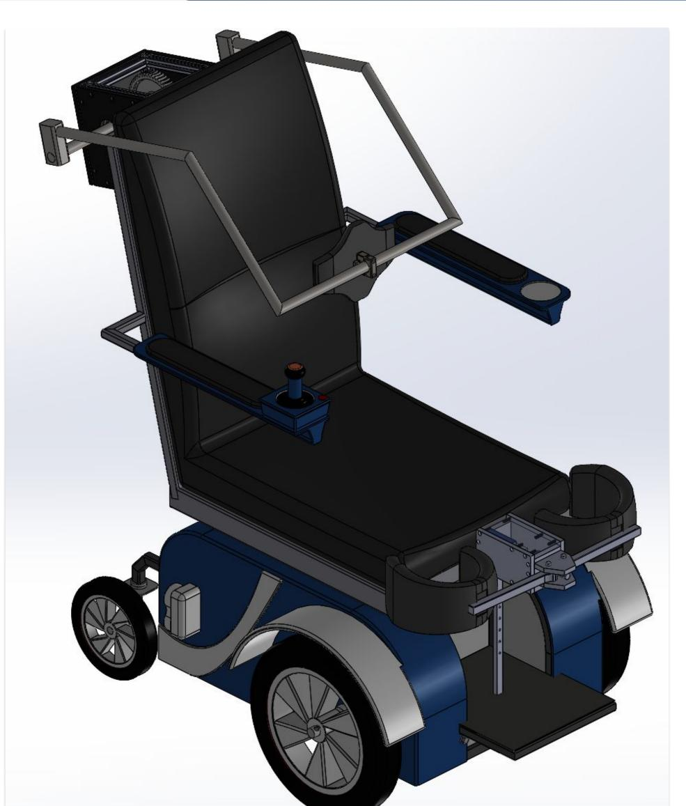
Figure 6: Overall Design Implemented on STS Wheelchair
