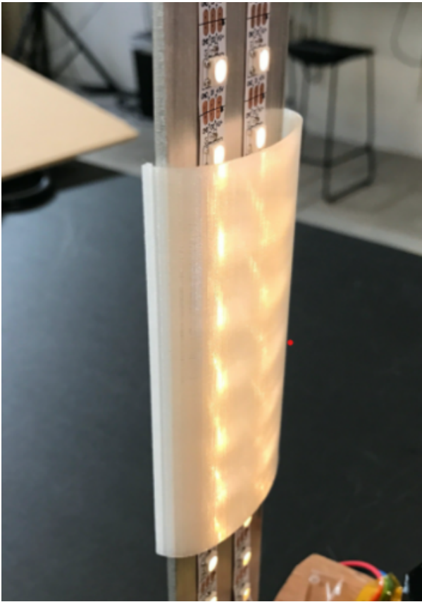
Figure 2. 3D printed LED diffuser clips
