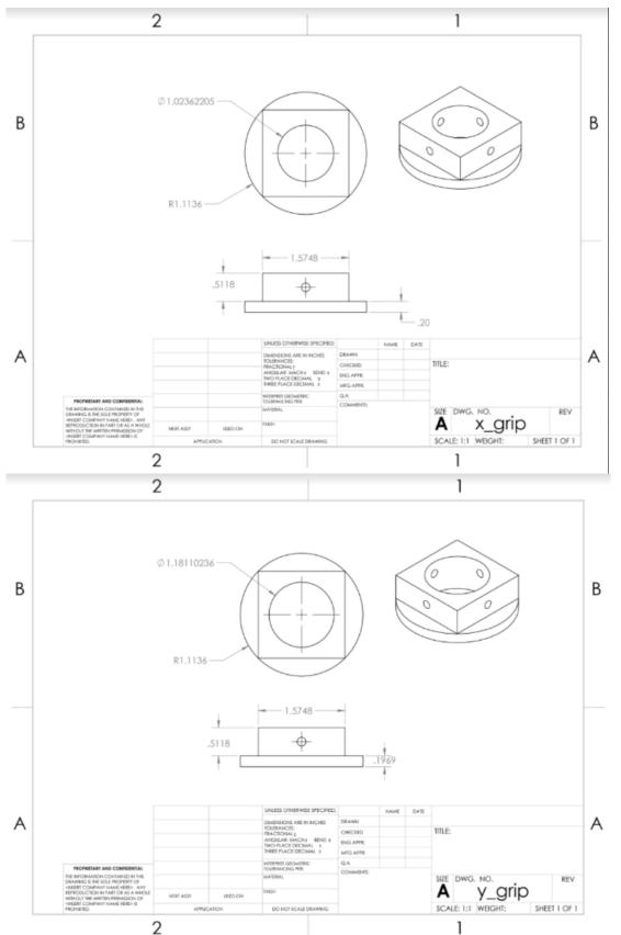
Two gear holders were fabricated, one for each knob. The only difference between the two gear holders was the diameter of the through hole, which matched the dimensions of the knobs that we wanted to fit.
