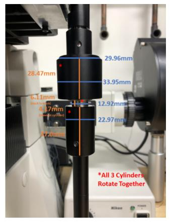
**Conclusions/action items:** These dimensions will be used to inform a SolidWorks drawing of a brace that will prevent pivoting of the control knob shaft during motor transmission.
