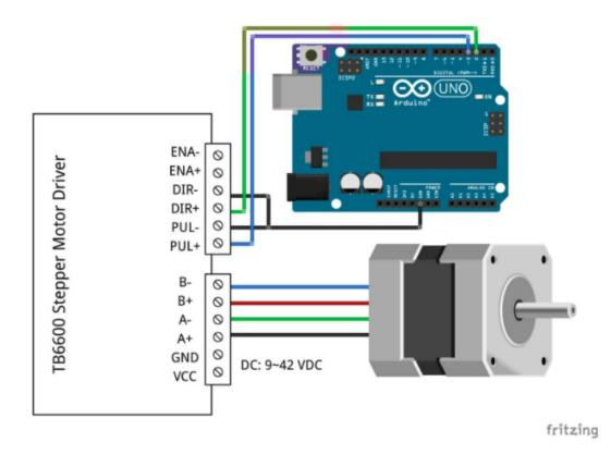
· Wiring schematic for the Arduino code we will be using (https://www.makerguides.com/tb6600-stepper-motor-driver-arduino-tutorial/)
