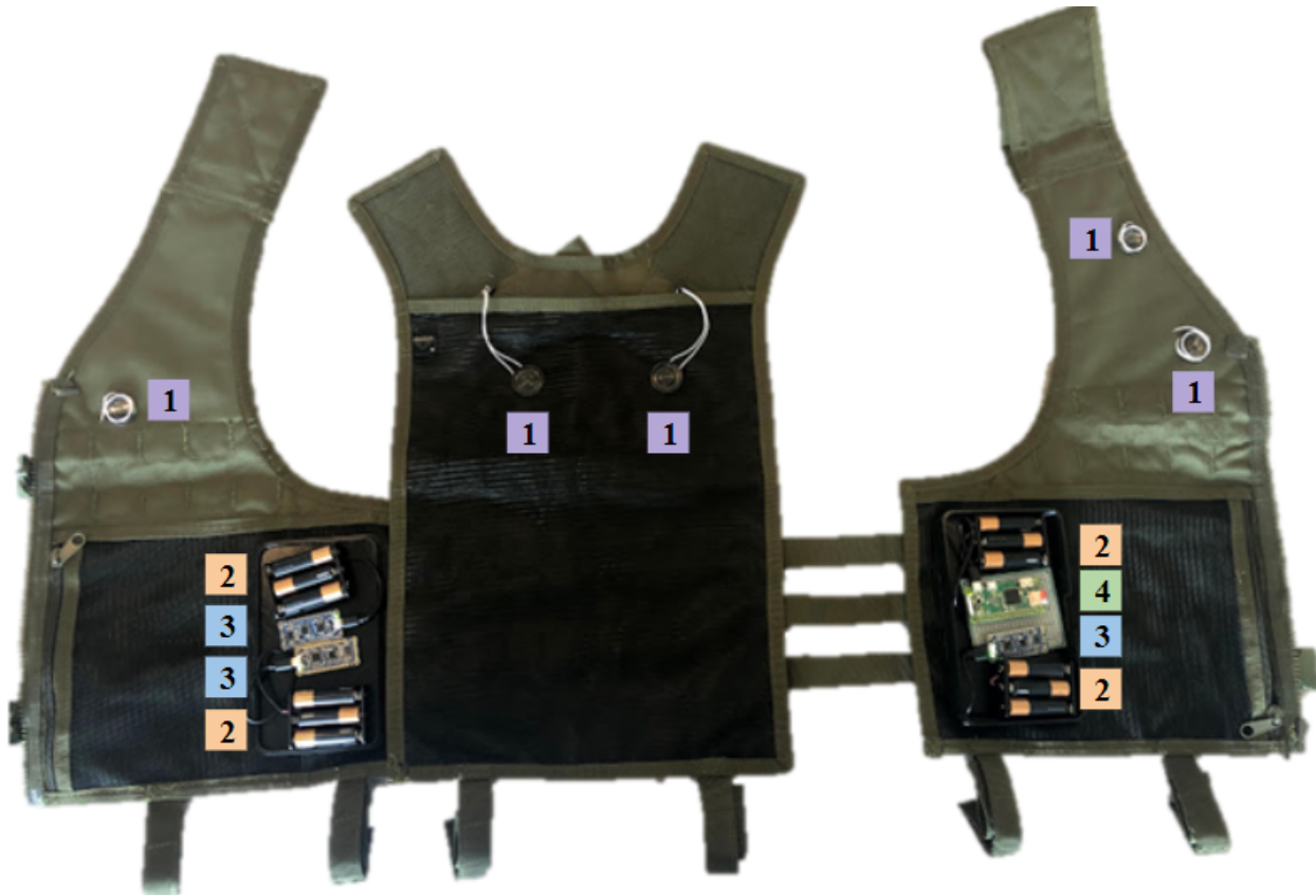
Figure 9: Hardware layout within vest. 1) The speakers are placed on the front and back to simulate heart and lung sounds. 2) Battery packs are used to power the 3) soundboards and 4) Raspberry Pi. Everything except the speakers is housed in plastic electronics boxes along the sides of the vests for protection. This is a view of the inside of the vest.
