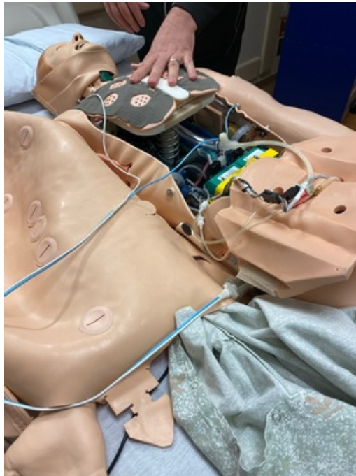
Chest_Area_of_manikin.jpg(156.6 KB) - download This is a picture of what is underneath the chest area of the manikin. Where the hand is in the picture is the chest piece of the manikin which rises and falls to simulate a normal (and abnormal) breathing. The manikin also generates breathing sounds which correlate to the rate of breathing occurring. There are also speakers on the breast plate which allow for one to listen the manikin's "heart" via a stethoscope. I do not think it can be seen in this picture but there are metal leads on the chest which also allow for the manikin to be connected to an AED and another device where one could actually change the different heart/lunge/pulse sounds/rates to correspond to a different situation; they specific wave and vital number are then displayed on the screen.
