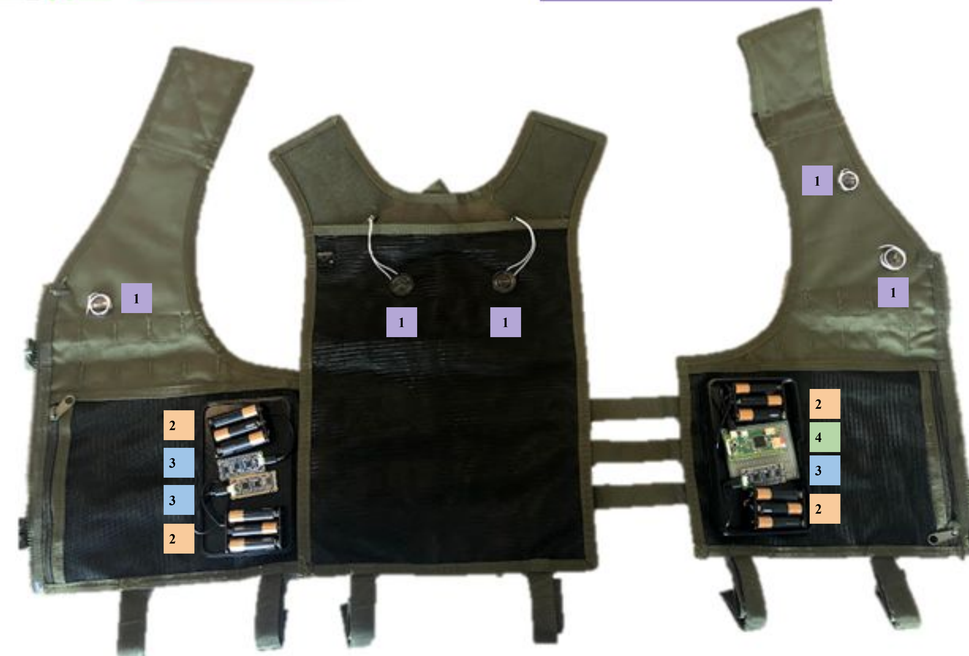
Figure 4: Hardware layout within vest. 1) The speakers are placed on the front and back to simulate heart and lung sounds. 2) Battery packs are used to power the 3) soundboards and 4) raspberry pi. Everything except the speakers is housed in plastic electronics boxes along the sides of the vests for protection.
