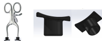
Figure 6: Adapted Weitlaner design (left), CAD model of the disposable rubber shod (right)
