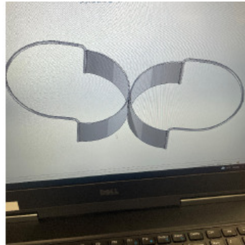
Figure 15: U Band Pincher design. The “pinchers” or clamp-like structures were scrapped early in the design process after concerns of difficult fabrication and obstruction of the procedure.
