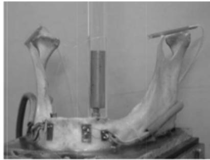
Fig. 3. Dynamic loading measurement set-up in the study
