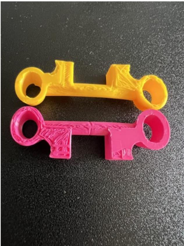
Figure 1: Final 2 models printed. Pink PLA incline plane fit best.
