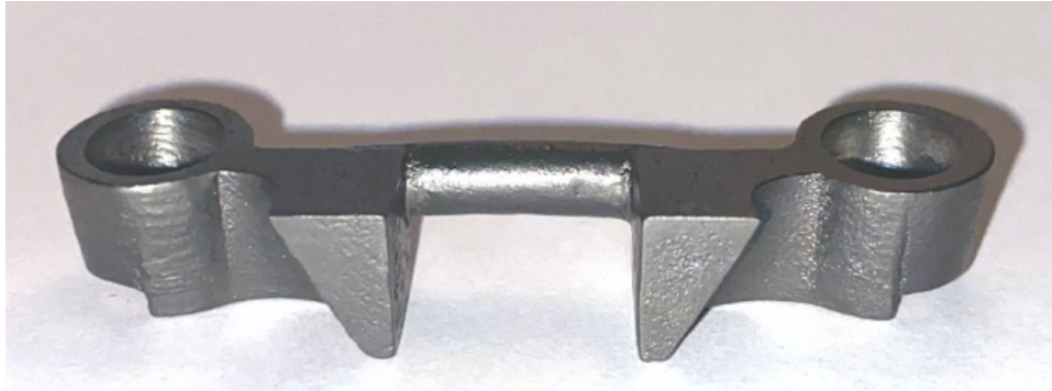
Figure 12: Front view of final prototype in Ti-64. This is the configuration for which it will be placed in the patient's mouth.
