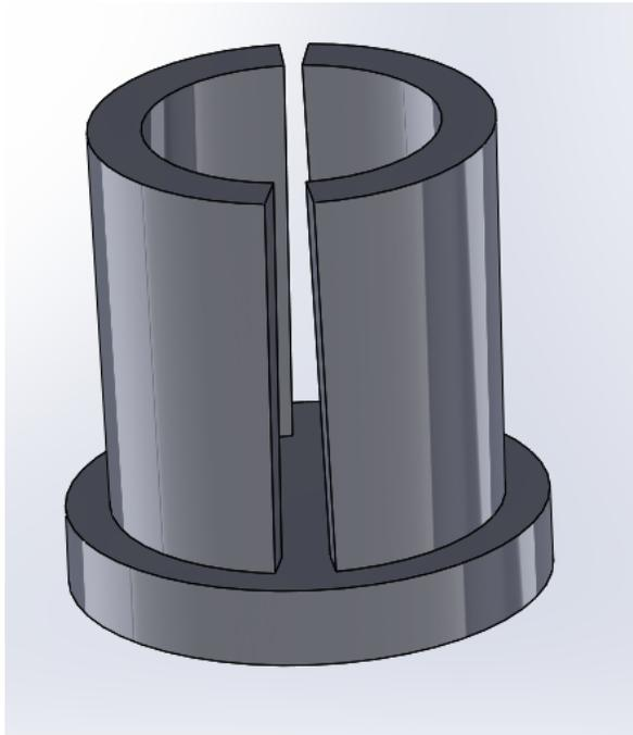
Other versions of the pin were printed with diameters of 4.7, 4.5, 4.3 mm to accommodate the poor tolerance of the 3D printers. The 4.5 mm pin fits and holds the retractor together the best.
