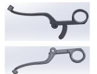
The left and right pieces of the retractor were modified to increase the length of the legs based on feedback from the ergonomics evaluation and cadaveric assessment. The locking mechanism was added directly to the right piece to increase the ease of assembly and prevent the use of an adhesive in the rapid prototyped models. The final design fabricated in stainless will still have these as separate parts.
