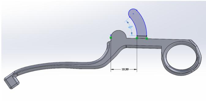
The left side of the model was updated so that the locking mechanism has a radius of 20 mm and an angle of 45 degrees.
