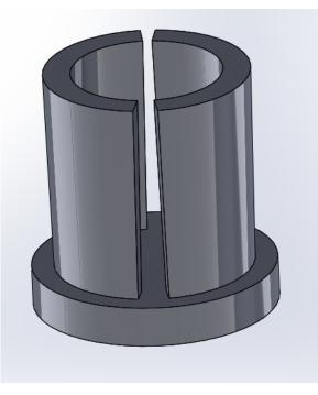
Other versions of the pin were printed with diameters of 4.7, 4.5, 4.3 mm to accomodate the poor tolerance of the 3D printers. The 4.5 mm pin fitsand holds the retractor together the best.
