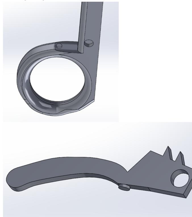
The right side of the device was modified to add a notch so that a spring may be added. The locking mechanism for the right side was also modified to allow addition of a spring.
