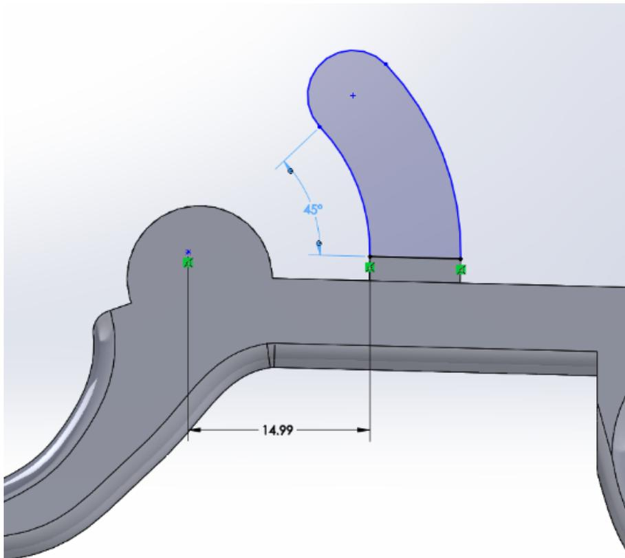
The locking mechanism on the left side of the model was updated to decrease the radius to 15 mm to increase the range of motion and reliability.
