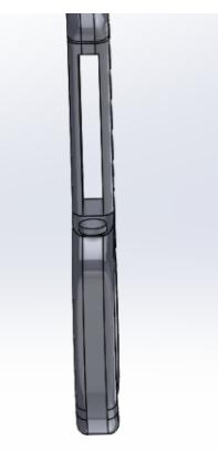
The right piece was modified to increase the diameter of the notch to better secure the spring. The length of the opening in the center was increased, to increase the range of motion as the locking mechanism passes through.
