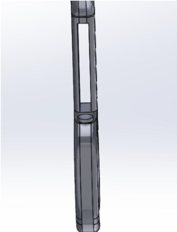
The right piece was modified to increase the diameter of the notch to better secure the spring. The length of the opening in the center was increased, to increase the range of motion as the locking mechanism passes through.
