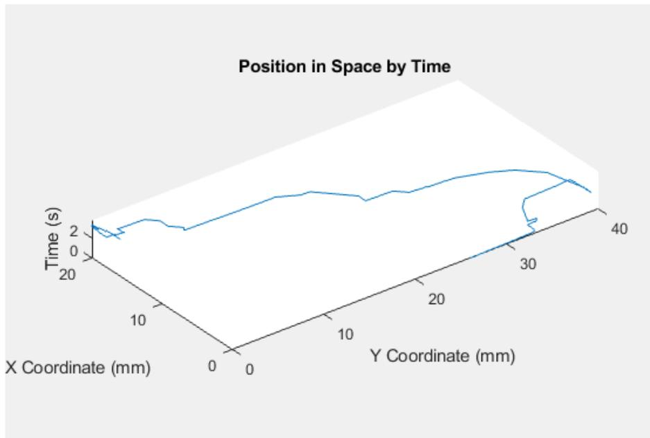
The code outputs the above plot of position in the xy plane vs. time, as well as the maximum force of 0.58 N and maximum acceleration of 2.9038 m/s<sup>2</sup>.
