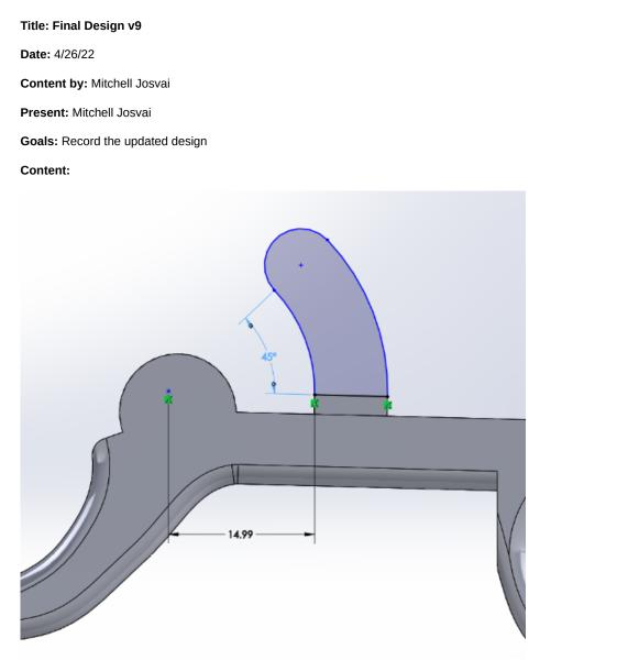
The locking mechanism on the left side of the model was updated to decrease the radius to 15 mm to increase the range of motion and reliability.
