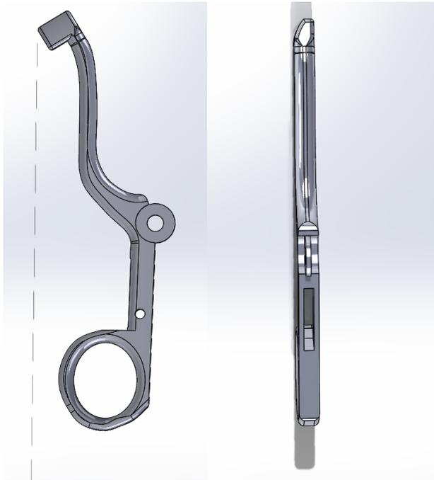
All fits together well with the 4.5 mm pin well. Still need to update the pins to screws and find a locking mechanism geometry that works
