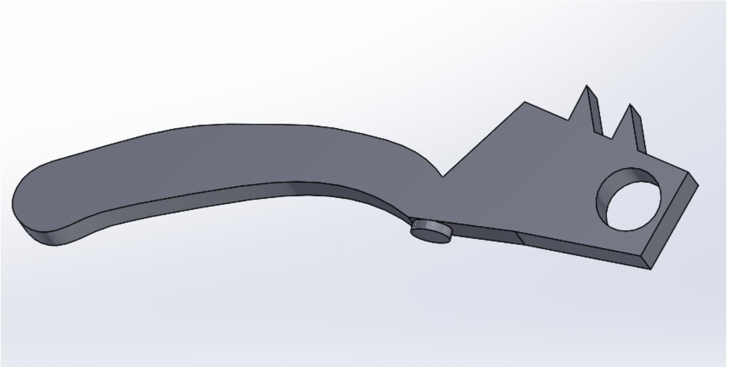
The right side of the device was modified to add a notch so that a spring may be added. The locking mechanism for the right side was also modified to allow addition of a spring.
