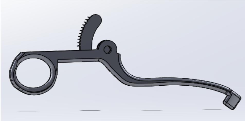
The design was updated to modify the gears to improve the reliability of the locking mechanism.
