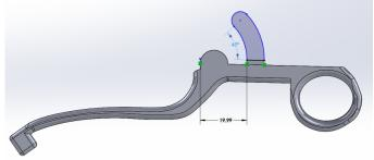
The left side of the model was updated so that the locking mechanism has a radius of 20 mm and an angle of 45 degrees.
