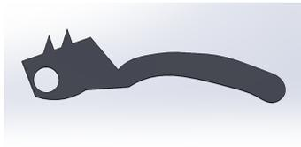
Locking mechanism part was updated increase the range of motion and prevent it from hitting the base of the retractor finger holes.
