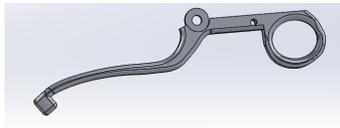
The left and right pieces of the retractor were modified to increase the length of the legs based on feedback from the ergonomics evaluation and cadaveric assessment. The locking mechanism was added directly to the right piece to increase the ease of assembly and prevent the use of an adhesive in the rapid prototyped models. The final design fabricated in stainless will still have these as separate parts.
