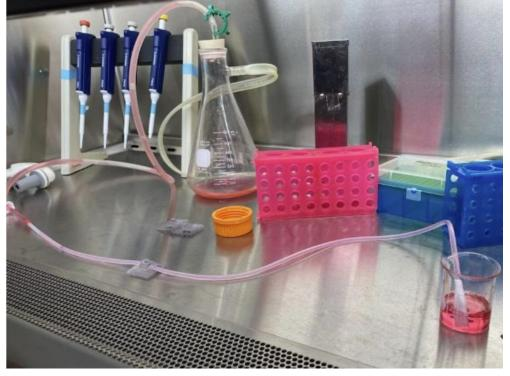
Figure 10: Flow testing was conducted on each clip iteration to determine if the clips impinged on the surgical drain, obstructing flow. A fluid with a viscosity similar to blood were conducted on each sample and was used to mimic the standard exudate of the rated based on how well the bandage drain. The vacuum in the biosafety cabinet appeared to be adhered. The rating scale was used to create a consistent flow.
